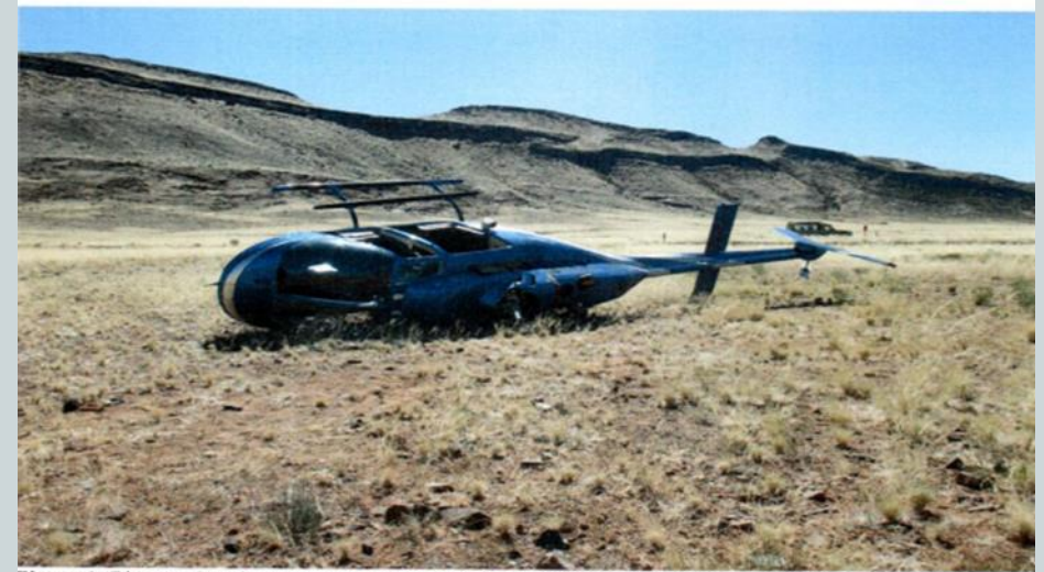
Figure 1: Picture showing damage to the aircraft especially to the main transmission system.
