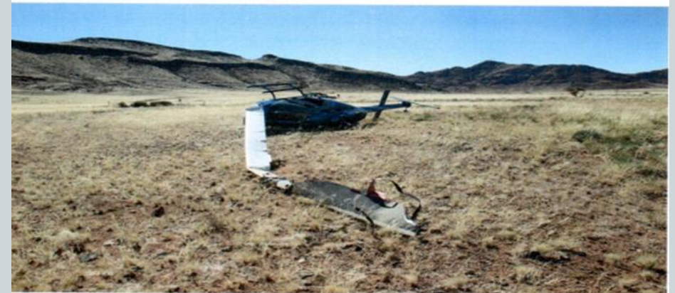
Figure 2: Picture showing the rotor head that broke off from the mast.
