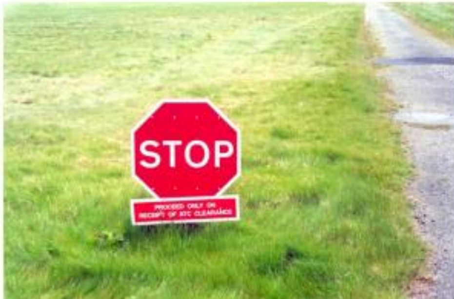
Figure 12. 41: Example of a road-holding position sign
