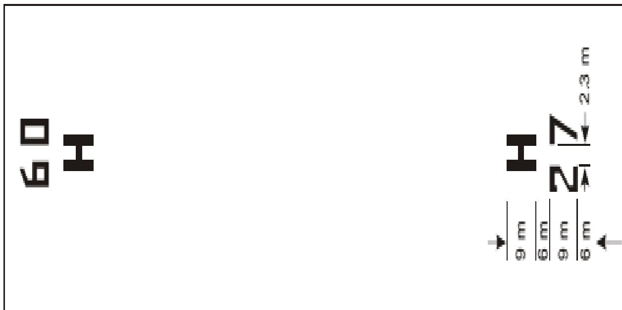
Figure 5-2. FATO designation marking and heliport identification marking for a runway-type FATO
